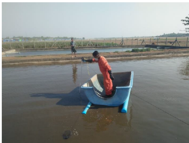
Figure 22: Measuring the quantity of sludge accumulated
