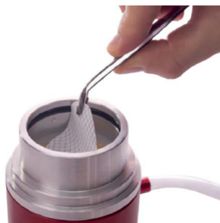
Figure 10. Use the sterile forceps to take the membrane from the filtration unit.
