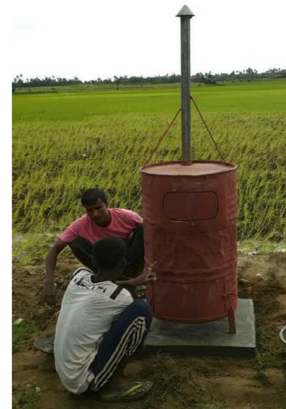
Figure 3. An incinerator bin built using a recycled oil barrel. Sanitary protection materials can be directly burnt inside by female environmental cleaners.
