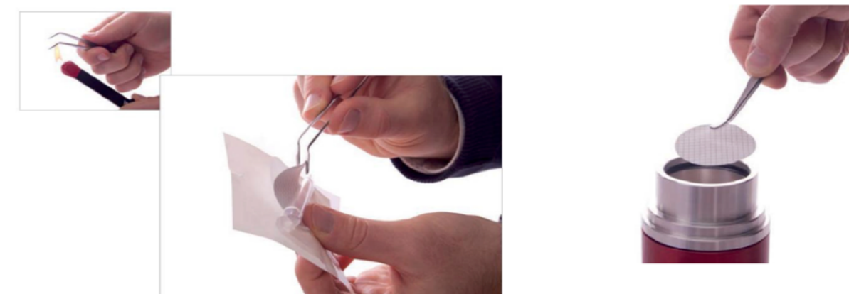
Figure 7. Sterilise the forceps and then place a sterile membrane onto the bronze membrane support.
