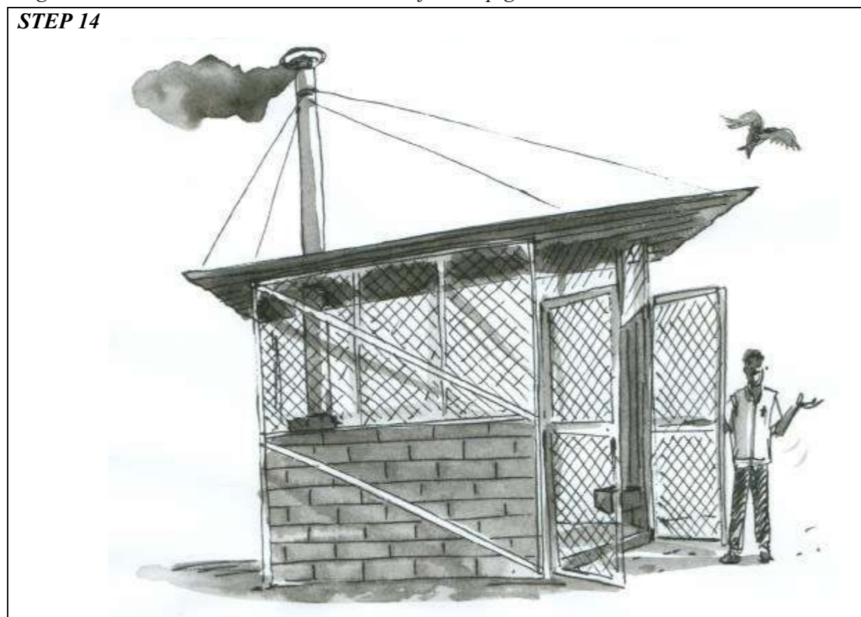
Figure 2.3.14 Finished WDU with chain link fence, spigot and ash door mounted
