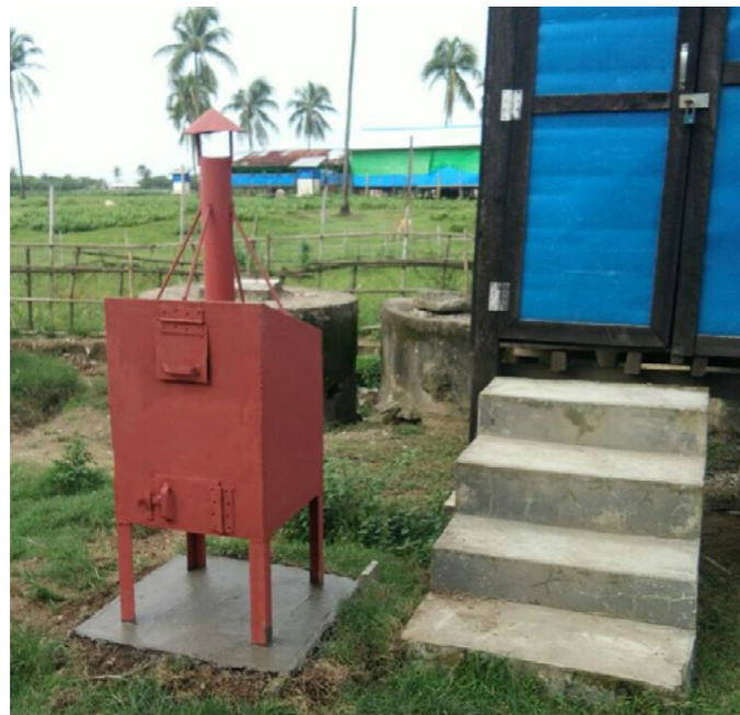
Figure 6. A rectangular incinerator bin designed by an ACE group in TKP
