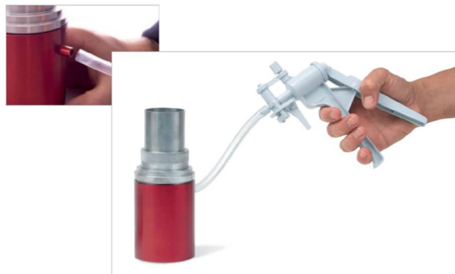
Figure 9. Apply hand pump to pass the water through membrane.
