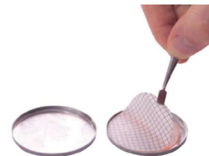
Figure 11. Place the membrane on top of the pad saturated with MLSB or CHROMAgar Liquid ECC.
