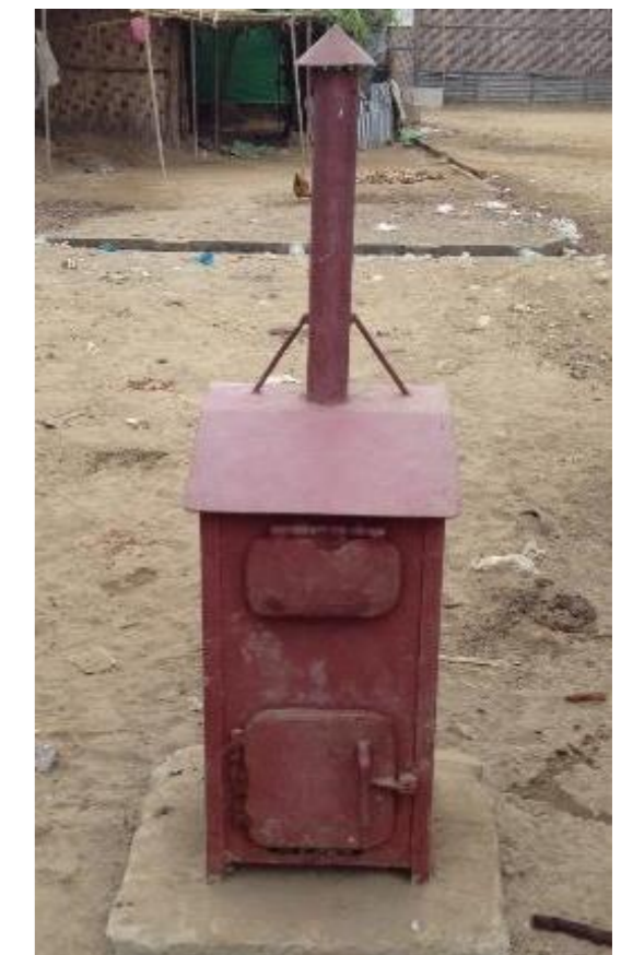
Figure 2. A smaller incinerator bin, only 1' x 1' x 3'.
