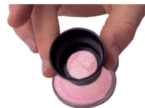
Figure 12. Count the yellow thermotolerant colonies (with a hand lens, if needed).
